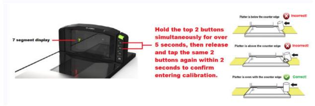
A 5-beep tone sequence will sound if calibration mode is successfully entered. Scan any configuration barcodes for things like changing the scale sensitivity at this time, then continue with the calibration.
